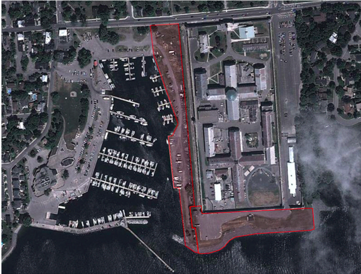
Figure 8. Satellite footage of Portsmouth Harbour and the former Kingston Penitentiary grounds. The shaded red area indicates the areas potentially affected by historical coal storage, according to CSC. After an ESA of the area was conducted in 2013-2014, soil in the shaded areas was excavated and large portions were paved over.
